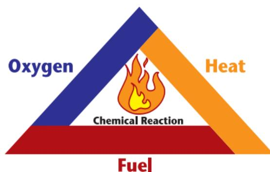
**5.7.4 Oxygen** — The most common source of oxygen is air, but oxygen can also come from chemicals called oxidizers. Examples of common oxidizers are some types of acids and chemicals such as chlorine, chlorine dioxide, potassium permanganate and potassium chlorate.
